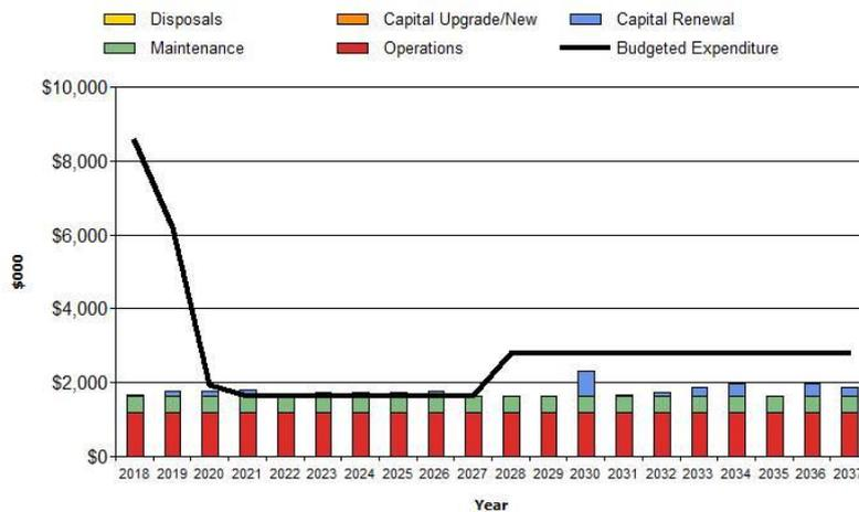
The Scenario 2 renewals are based on technical judgement made by staff as to the works required to be completed to maintain current service levels. As shown in the diagram below the capital budget has only been completed for the first three years, as this is refined more we can expect the costs to rise above budget expenditure in some years.
