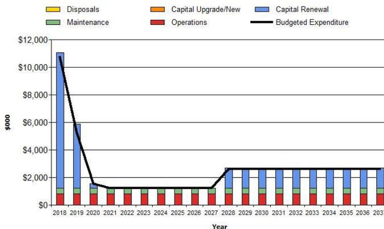
The below graph shows scenario 3 with a balanced graph with the expenditure figures balanced out to match the available budget. The capital budget has only been developed for the first three years as it is further developed it will be included in this plan.
