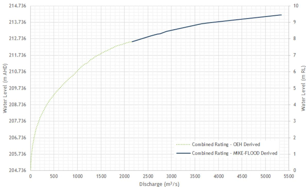
Figure 5.1 - Adopted combined high flow rating curve Narrabri Creek at Narrabri (GS419003)
